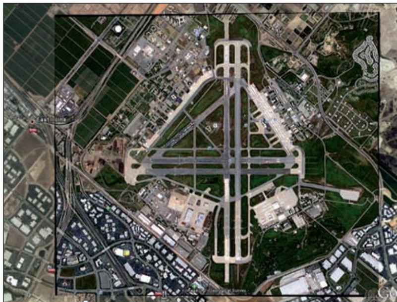
Figure 3: Full resolution orthorectified RapidEye image of Irvine corrected without GCPs overlaid with Google Earth
