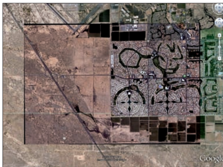
Figure 5: Full resolution orthorectified RapidEye Phoenix data corrected without GCPs overlaid with Google Earth
