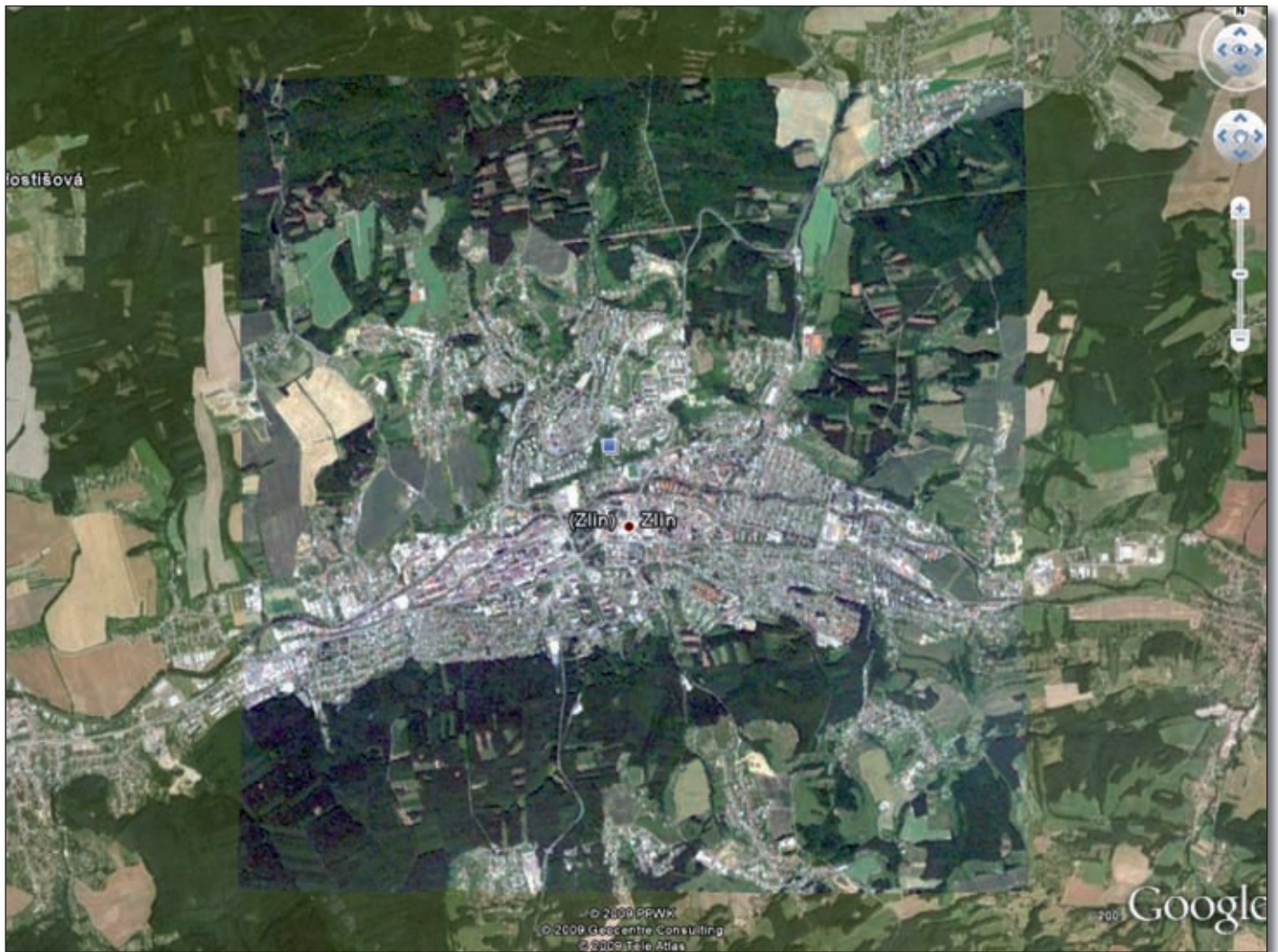
Figure 6: Full resolution orthorectified RapidEye Zlin data corrected without GCPs overlaid with Google Earth
