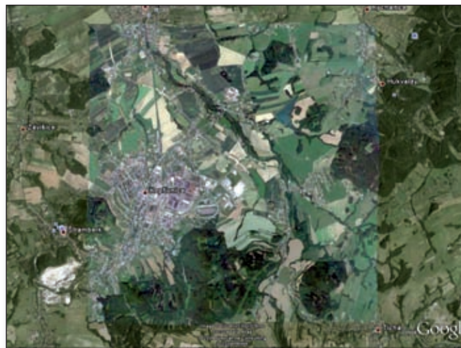
Figure 7: Full resolution orthorectified RapidEye Koprivnice data corrected without GCPs overlaid with Google Earth
